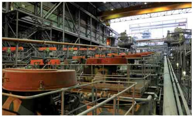
Flotation cells at BRPM's concentrator
